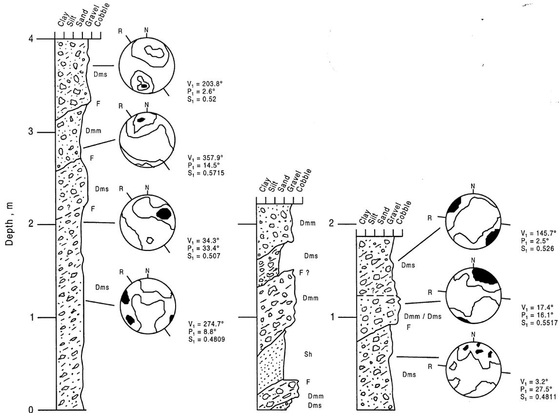
Figure 5. Graphic sedimentary logs of sections in the thrust-block moraines. The contour interval of the Schmidt nets is two standard deviations.  $V_1$  and  $P_1$  give the azimuth and plunge of the principal eigenvector, respectively, and  $S_1$  gives the strength of clustering about the principal eigenvector.
